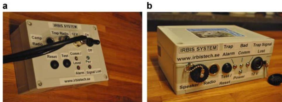
**Figure 2.** Key components of the Irbis System: (a) monitor unit and (b) camp unit. These electronic units are custom designed for the Irbis System, operate from 12-V DC power supply, and are moisture- and dustproof.
